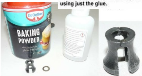
Pic 3. Glue the halves back together using just the glue.
