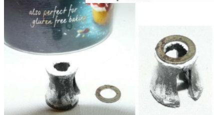
Pic 4. Pile some fine powder onto the top of the spacer, then lay the reinforcing washer on the powder.
