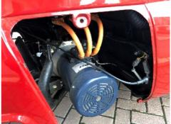
The project was a bit of a challenge as the three-wheel design is a little unstable and the Tesla motor is quite heavy. In fourwheel drive cars you don't have to worry about balancing the weight but this was an issue for the Isetta. Working out how to drive the rear wheel was also a bit of a challenge.
