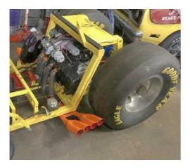
To fit the tube frame and tyres, the rear of the Isetta's body has been widened by 10 inches (all fabricated in metal). It has a 6-speed gearbox driving a narrowed Ford 8" rear axle into a custom golf cart chain drive rear. For ultimate Dragster authenticity it has long "Wheelie Bars" at the back to keep the front wheels on the asphalt, and a huge rear wing to complete the picture. Just for effect, it has four exhaust pipes exiting each side.
