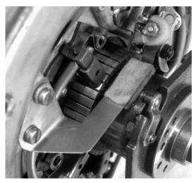
top of the cam oiler. Use screws no longer than 5mm so you are certain you will not hit the armature windings? At the dashed line where it says "bend up', make a 90° bend using a small vice.
