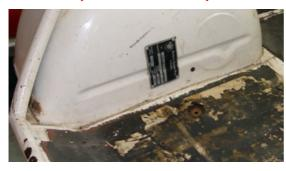
The condition of the floor is very important. Any holes or pop riveted repairs are unacceptable, on roadworthy car at least. If there are bodged and have an un-ribbed panel welded in you will suffer extreme drumming, due to vibration. The area of floor where you step in flexes a lot. Add to this moisture and dirt trapped under the rubber floor mat and the floor can go very thin. Check along the joint between the floor and the inner
