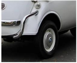
the inner and outer panels were welded together. Moisture, dirt and debris collect in the joint, inside the car and out and start to push the panels apart. Repair is tricky, but the Club do have inner arch repair panels made.
