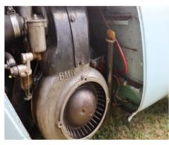
The main reason for the big end going is of course lack of oil. The slinger ring (Exploded view No.1 part No.37) is the culprit. It fills up with debris and eventually cuts off the oil supply. If you are doing a full rebuild make sure you clean it out and change your oil regularly.
