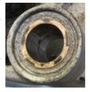
15 Insert the suspension arms and again look for a tight fit with no lateral movement – if it does you may have to have new shell bearings made which have extra thickness and the arm refaced to match!
