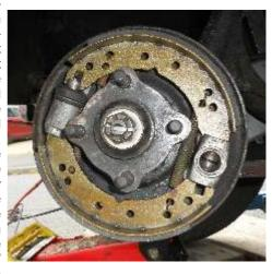
this the leading shoe, however when you operate the hand brake with the car rolling backwards you want the brake to grab easily and hold the car so the lining material is set next to what has now become a leading edge.
