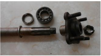
It is worth noting the slotted bearing spacer has an internal taper mating with the machined flange on the axle and the flat side of the spacer abuts to the rather special 22205C3 bearing. These double row self aligning ball bearings are rather expensive so be very careful when trying to save money
