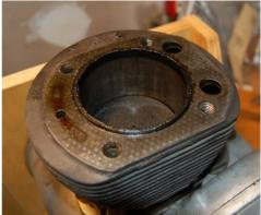
. I looked into the empty barrel, thinking maybe there would be evidence of an escaped circlip. The sidewalls of the cylinder told the story, two deep grooves on each side of the piston from the hardened pin rubbing up and down the cylinder walls.
