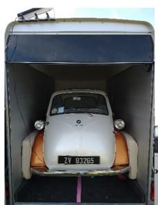
ble horse power. The rear door of the trailer can open either sideways, for access inside or downwards to form a ramp for loading and unloading the car.
