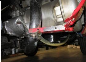
22. Disconnect the brake light switch wires (from underneath car from front) Green to Right and Red to Left side of switch.
