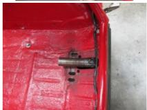
33. Remove the 4 bolts holding the towing eyes and Cow Catcher bars to front of vehicle at the floor.
