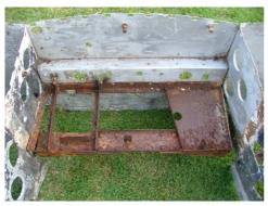
inner wings. The bulkhead had so many holes in it I decided to remake that also. The inner wings required large flared holes to be formed in them to allow cooling air to escape from the engine bay.
