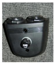
Note the inline fuse I added which is accessible from the front!
