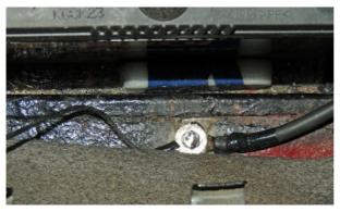
The strap from the engine to the chassis had had good contact. The one from the battery to the floor was a different Kettle of Fish. (If yours is like mine the earth strap goes to the floor of the Isetta and connects to the chassis through a 10mm captive nut. In my Isetta it's hidden under the carpet!)
